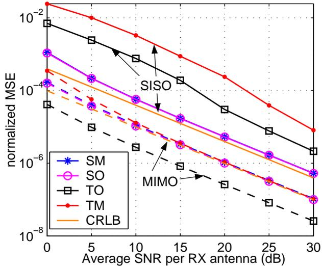
Fig. 7. MSE in CFO estimation (normalized to the subcarrier spacing) for different preamble formats as function of the SNR for a SISO (—) and  $4 \times 4$  (---) system and a rms delay spread of 10 ns.
