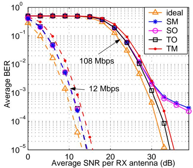
Fig. 8. BER performance of a  $2 \times 2$  system applying the different preamble formats. Results are given for BPSK, rate 1/2 coding (12 Mbps) and 64-QAM, rate 3/4 coding (108 Mbps).
