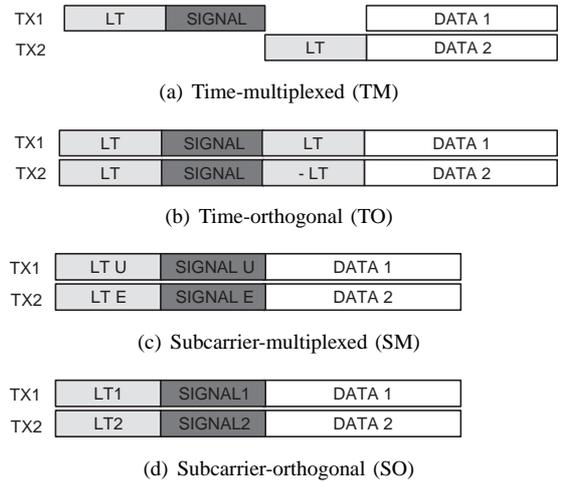
Fig. 2. Backwards compatible MIMO PHY frame formats.
