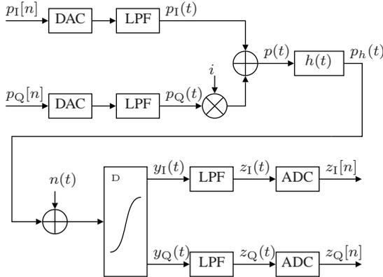
Fig. 2. Baseband equivalent system model for the transmit and receive chain.
