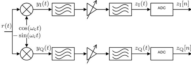
Fig. 1. System model for a non-impaired down conversion receiver
