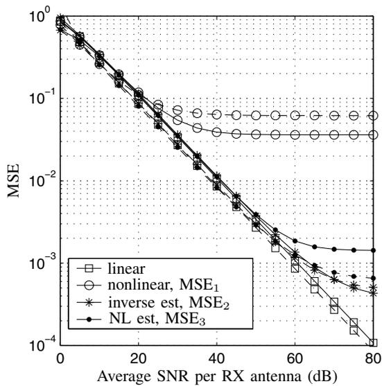
Fig. 2. MSE for a  $2 \times 4$  system with perfect (dashed lines) and estimated (solid lines) MIMO wireless channel knowledge.
