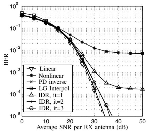
Fig. 3. BER results for a  $2 \times 4$  64-QAM system applying different RX-based nonlinearity correction methods.
