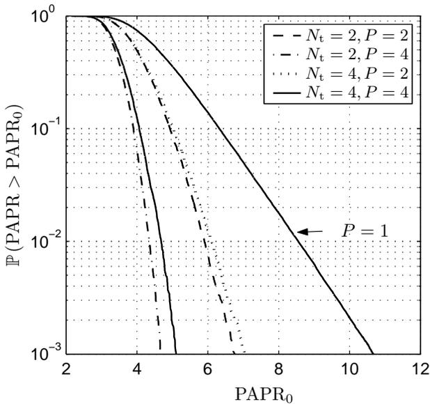
Fig. 3. CCDF of the PAPR for the combined SS/PS method for the PR subcarrier grouping scheme.
