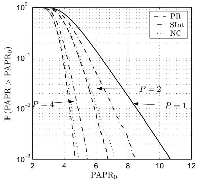
Fig. 5. CCDF of the PAPR for the combined SS/PS method for the different subcarrier grouping schemes, for  $N_t = 2$ .
