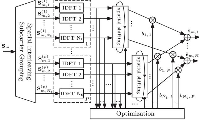
Fig. 1. Block diagram of a MIMO OFDM TX combining SS and PS.
