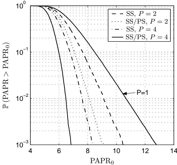
Fig. 6. CCDF of the PAPR for the transparent SS and combined SS/PS method for the PR subcarrier grouping scheme, for  $N_t = 2$  and  $M = 10$ . PAPR is calculated for the entire 10 OFDM symbol packet.
