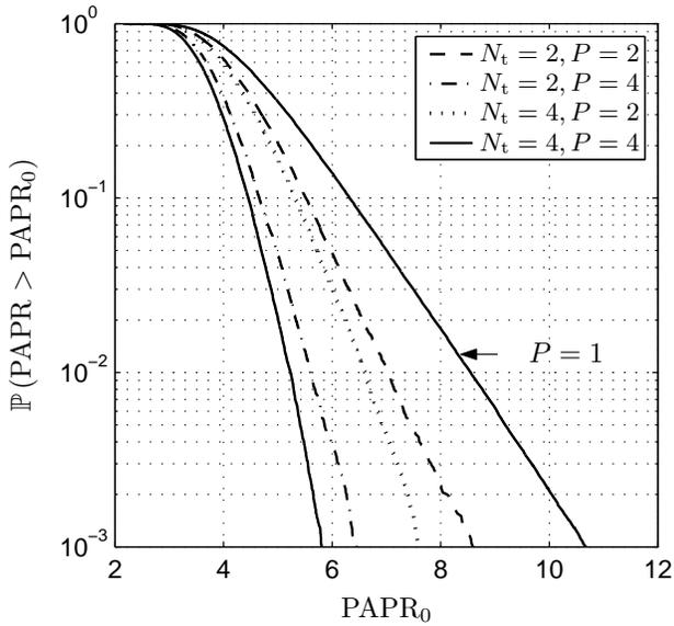
Fig. 2. CCDF of the PAPR for the SS method for the PR subcarrier grouping scheme.
