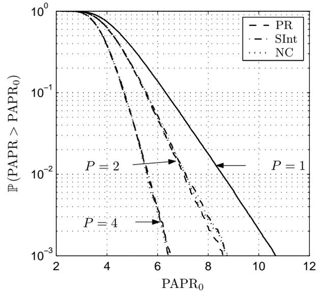
Fig. 4. CCDF of the PAPR for the SS method for the different subcarrier grouping schemes, for  $N_t = 2$ .
