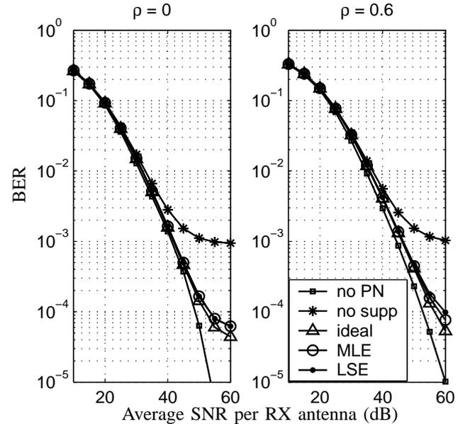
Fig. 4. BER for a  $2 \times 2$  ZF receiver for no PN, no suppression and ideal, MLE and LSE based CPE correction.  $P_{pn} = -24$  dBc and  $f_c = 100$  kHz, 5 OFDM symbols per packet,  $\rho = 0$  and 0.6, flat Rayleigh fading.
