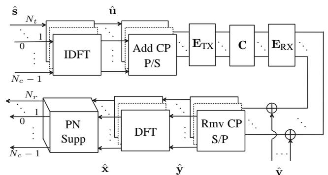
Fig. 1. MIMO OFDM system model with TX and RX PN impairments and PN suppression.
