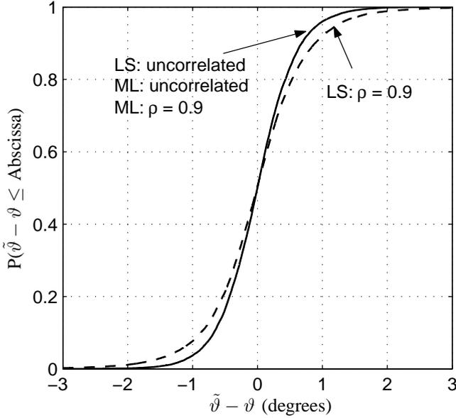
Fig. 2. ECDF of the error in estimation of  $\vartheta$  for a  $2 \times 2$  configuration,  $P_{pn} = -30$  dBc and  $f_c = 200$  kHz, 20 symbols per packet,  $\rho = 0$  (uncorrelated case) and  $\rho = 0.9$ , independent Rayleigh fading.
