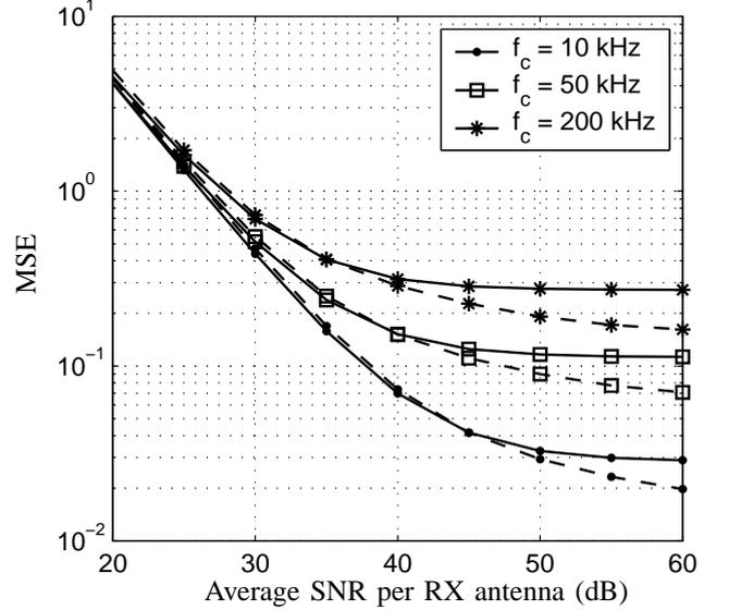
Fig. 3. MSE in estimation of  $\vartheta$  (in degrees) for a  $2 \times 2$  configuration for MLE (—) and LSE (---),  $P_{pn} = -30$  dBc, 5 OFDM symbols per packet,  $\rho = 0.7$ , flat Rayleigh fading.
