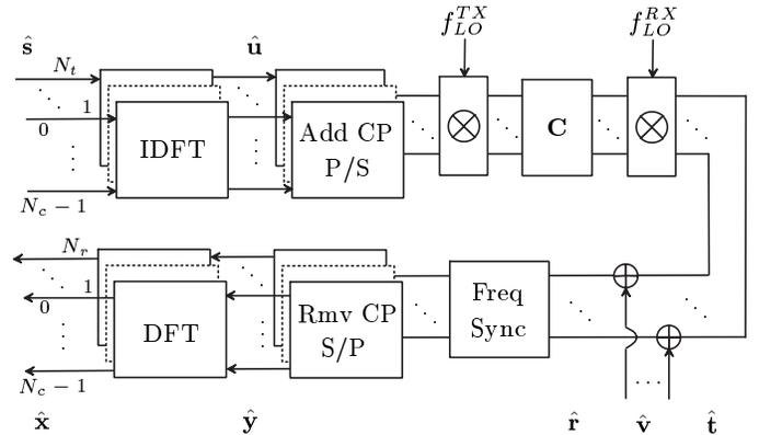
Fig. 1. MIMO OFDM system model with frequency synchronization.
