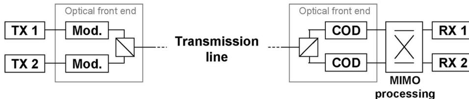
Fig. 1. Concept of PDM enabled by MIMO processing at the receiver, with TX =baseband transmitter, Mod.=Modulator, COD=coherent optical detector, and RX =baseband receiver.
