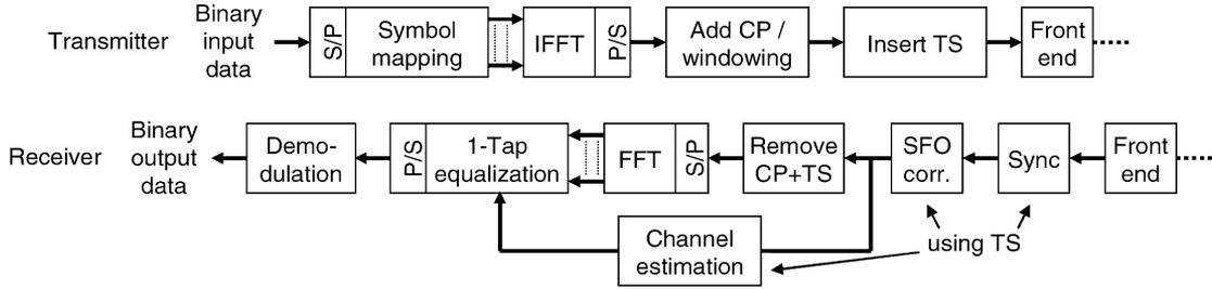
Fig. 1. Block diagram of a typical OFDM transmitter and receiver, with CP = cyclic prefix, TS = training symbol, Sync. = Symbol Synchronization, SFO = sample frequency offset, P = parallel and S = serial.
