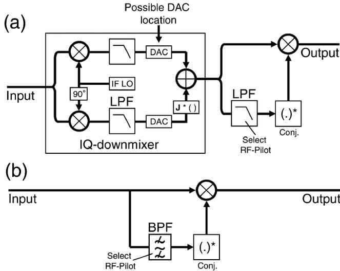
Fig. 3. Two possible implementation for downconversion from the IF into the baseband and phase noise compensation.
