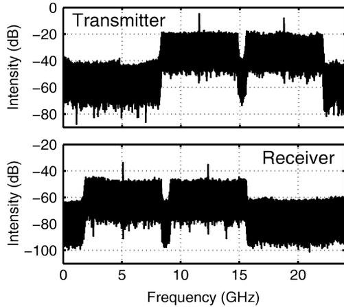
Fig. 7. Electrical spectra at a 10-MHz resolution bandwidth. (a) At the transmitter after multiplexing the two 12.9-Gb/s OFDM bands together. (b) After heterodyne detection with a balanced photodiode.
