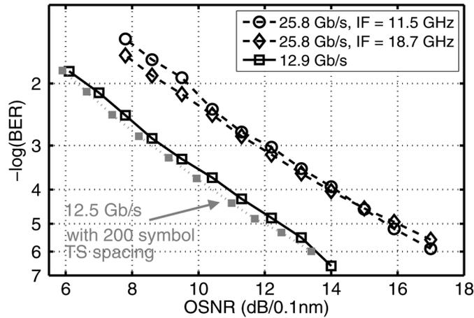
Fig. 10. BER as a function of the OSNR in back-to-back configuration.
