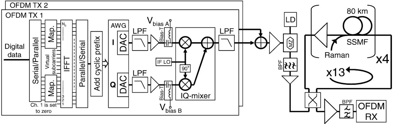
Fig. 5. Transmitter and transmission line of the experimental setup.
