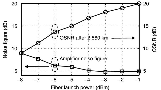
Fig. 12. Noise figure of the EDFA/Raman combination and the OSNR after 2560-km transmission as a function of the fiber launch power.
