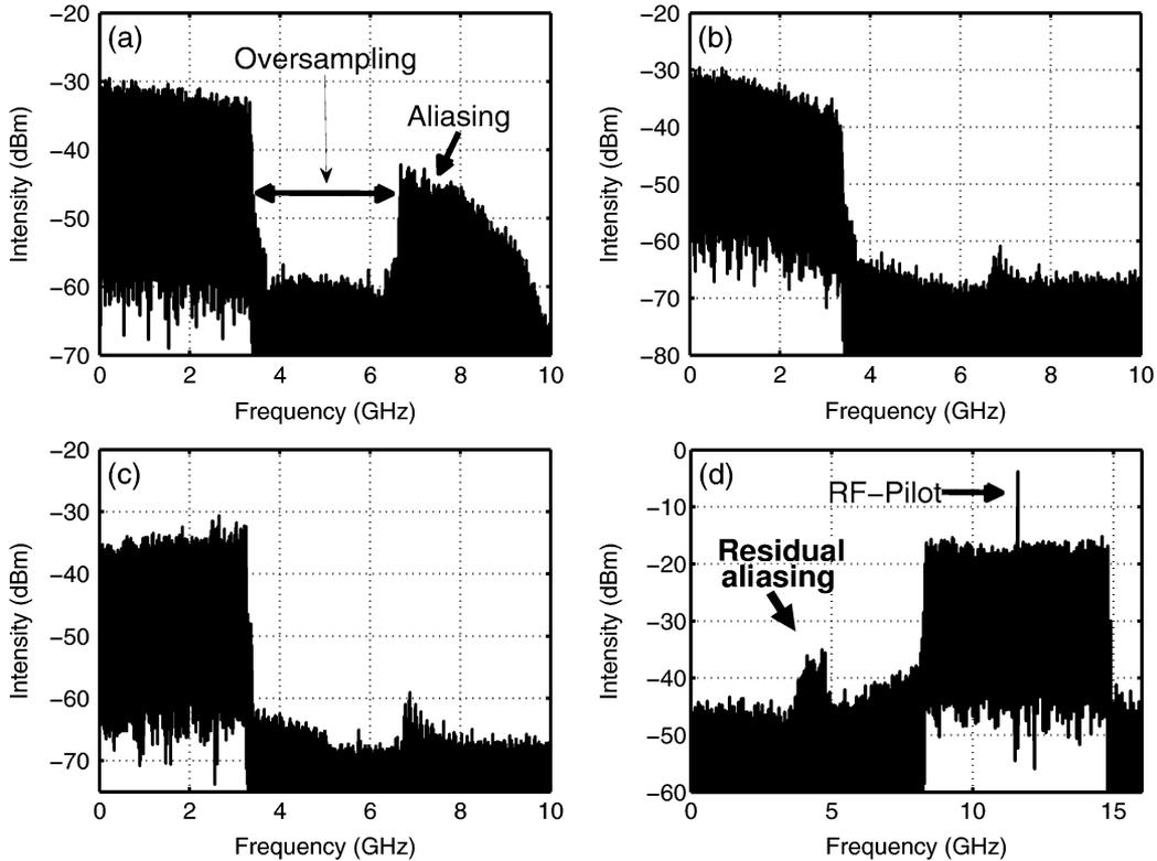
Fig. 6. Electrical spectra at a 10-MHz resolution bandwidth. (a) AWG output. (b) AWG output after LPF. (c) AWG output after LPF with preemphasis. (d) IQ-mixer output with preemphasis.
