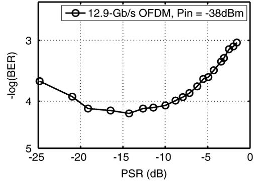
Fig. 4. BER as a function of the pilot-to-signal ratio (PSR).
