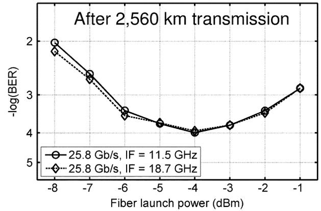
Fig. 11. BER as a function of the fiber launch power measured after 2560-km transmission.
