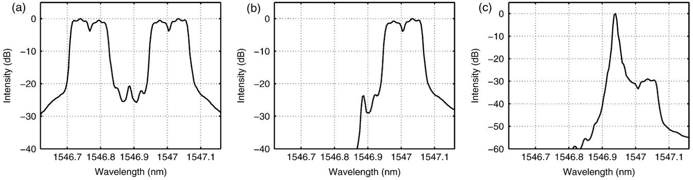
Fig. 8. Optical spectra at 2.5-GHz resolutions bandwidth. (a) After modulation. (b) After SSB filtering. (c) At the receiver just before the balanced photodiode.
