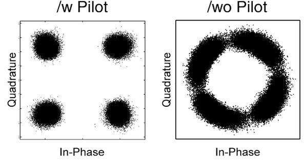
Fig. 2. Vector constellation diagram with and without RF-aided phase noise compensation (overlay of all subcarriers).
