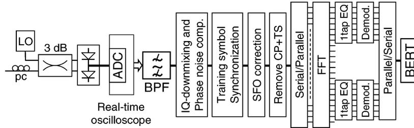
Fig. 9. Experimental setup of the heterodyne detector and software implementation of the OFDM receiver.
