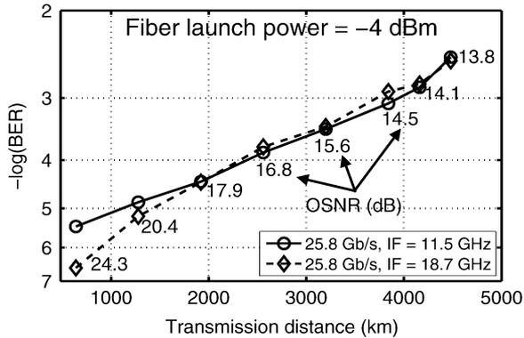
Fig. 13. BER as a function of the transmission distance for a fiber launch power of -4 dBm.
